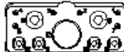
13P1 2 x Size 12 Contacts 4 x Size 15 or 16 Contacts 6 x Size 20 Contacts 1 x Size 5 Power Contacts
